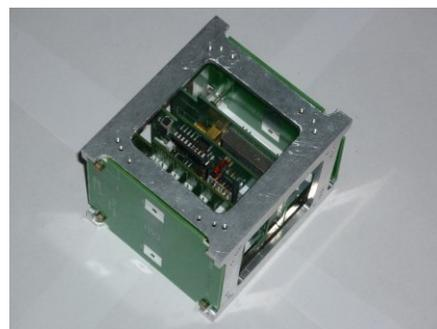
The total mass of the basic CubeSat systems is 0.65 kg. This leaves 0.35 kg or 0.68 for your experiment or application. (Total 1.00-kg or 1.33-kg options)
